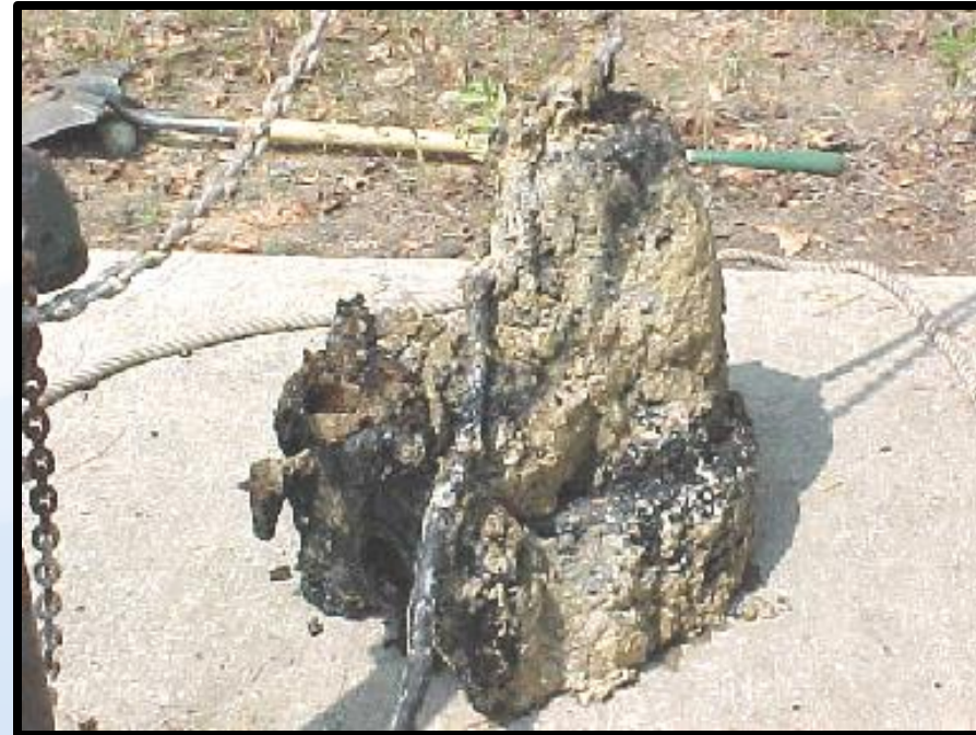
Grease build-up on submersible pump in lift station
