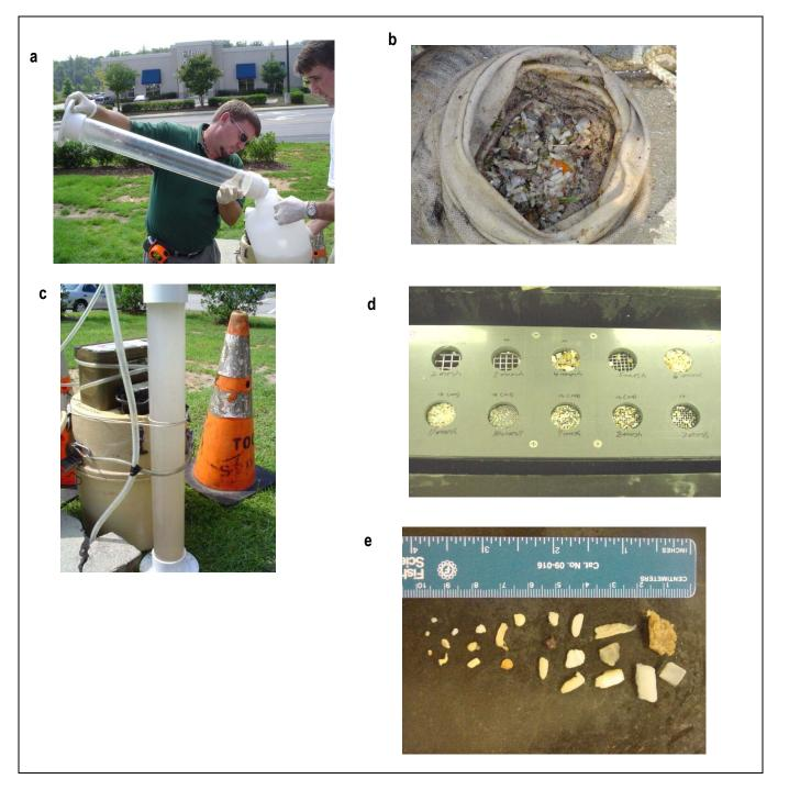
Figure 4-1. Solids Capturing and Measurement: a) Suction Chamber, b) Sock Capturing Device, c) Automatic Pump and Sampling with Suction Chamber, d) Stainless Steel Mesh Table, e) Image of Particles.
