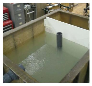
Figure 2-3. Pilot Scale Grease Interceptor.
