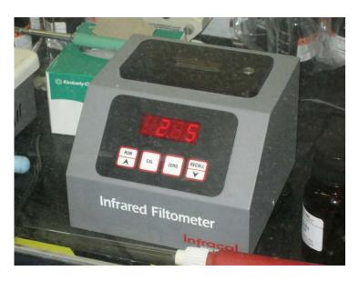
Figure 2-10. Infracal® Device Used for FOG Concentration Measurements.
