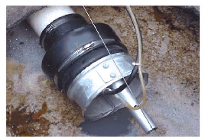
Figure 2-1. V-notch ISCO/Teledyne Flow-Poke Flow Measurement Device in Gl.
