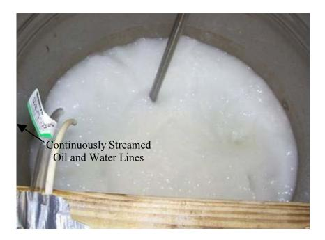
Figure 2-5. Oil/Water Mixing Drum.
