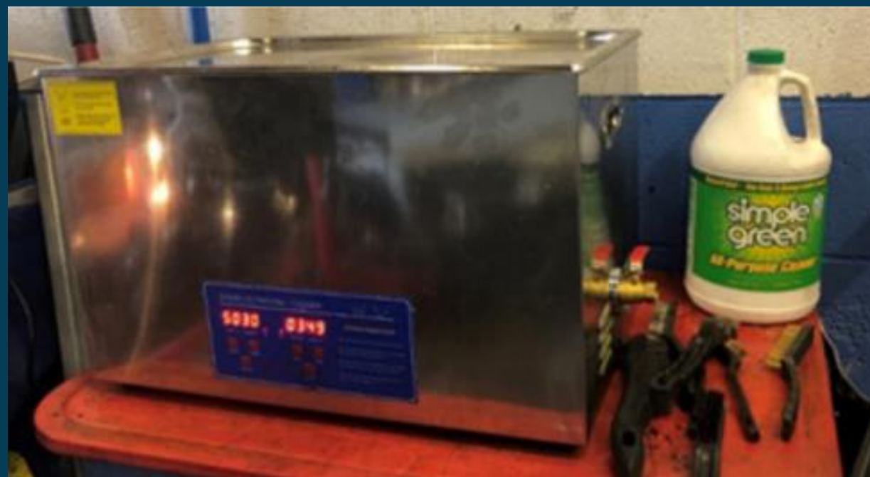
Ultrasonic parts cleaner and Safer Choice Simple Green All-Purpose Cleaner
